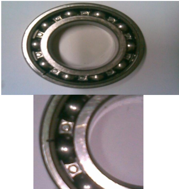
Figure 4.1(a): Outer race defect: Axial groove on inner surface of the outer race
