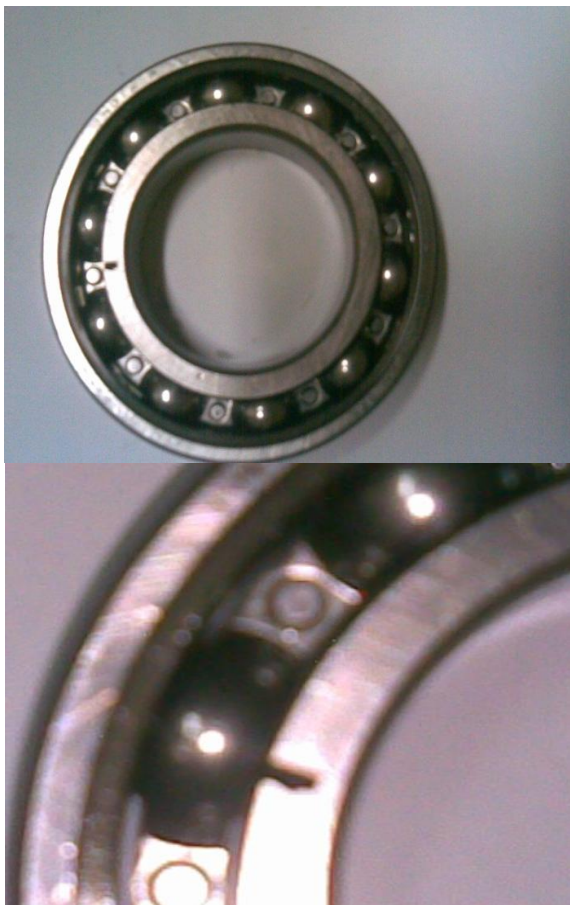
Figure 4.1(b): Inner race defect: Axial groove on outer surface of the inner race
